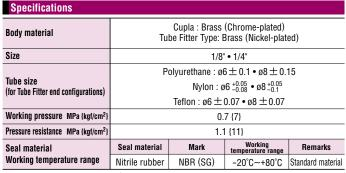
Above specifications apply only to Cuplas. Working pressure, pressure resistance and working temperature range may vary depending on tube materials you use with and temperature conditions you use under.
